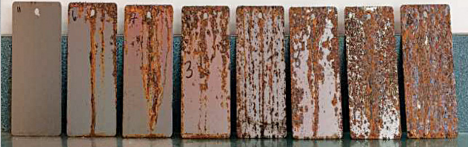
CorrosionX XD (far left) versus competitors after 120 hours in salt spray test
